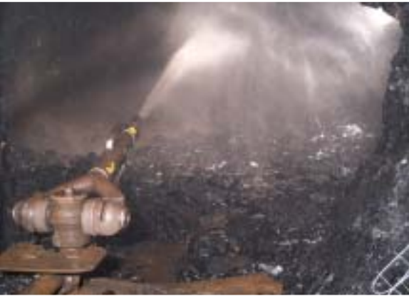
Left: Hydraulic monitor, underground; Right: The roadheader used underground.
